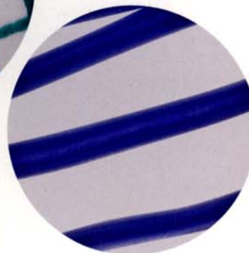
C. At 50X magnification, these reinforced adhesive strands show a metered amount of adhesive applied to its reinforced core. This allows for a predetermined amount of reinforced adhesive.
